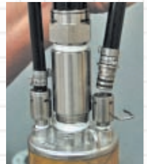
Once the clips are removed, simply pull the connections apart.
