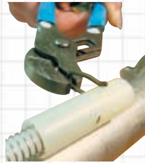
Removing the spring clip allows for easy disassembly of the float.
